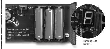
2. Confirm that a short beep sounds when a key is pressed and the number or letter of the key pressed is displayed on the numeric LED display.
